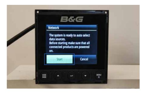
A progress bar will be shown to let you know it is looking for devices connected to the NMEA 2000 network. In this picture below, the B&G is recognizing the NCP High-End. If you B&B display does not recognize your NCP High-End please double check the connection. If the issue persists, contact us at *sales@calypsoinstruments.com.*
