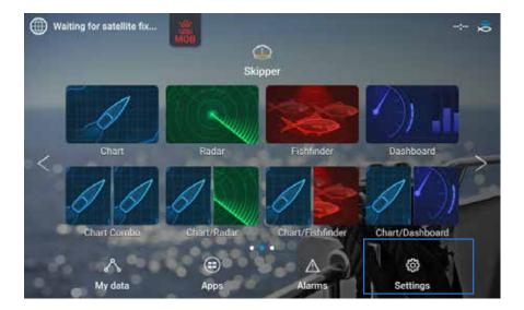
Once in settings, press on **Network.** Make sure your NCP High-End appears in this section as it means it is connected. If for some reason you don't see it, it means the NCP High-End is not being detected by the Raymarine display. Please double check your connection. If the issue persists, contact us at **sales@calypsoinstruments.com**.
