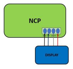
1. Connect to the terminals of the **N2K** on the bottom right corner as observed in the photo. In this case it is not necessary to have an external power supply as the N2K provides the power.
