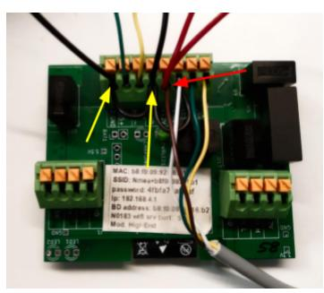
6. Wired Ultra-Low-Power RS485 wind sensor to NMEA2000 Display/Backbone
