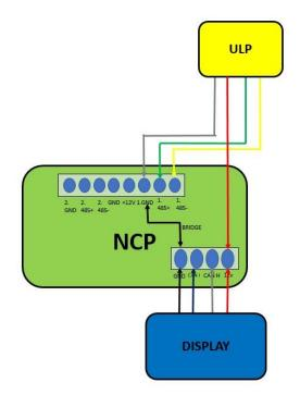
\* A bridge is a connection between two ports as shown in the graph above.
