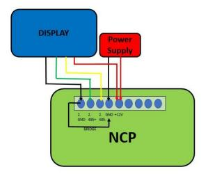
1. For the device to work, we will need to connect it to an external power supply of 12 Volts. The positive terminal of the energy source goes to the pin +12V of the ports of the top terminal as seen in the image. The negative terminal of the energy source connects to the GND. The green light should be lit. If it is not, check that the cables are properly connected. Before continuing any further, turn off the power to the energy source, do not disconnect the cables.
