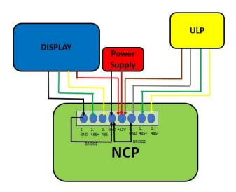
\* A bridge is a connection between two ports as shown in the graph above.
