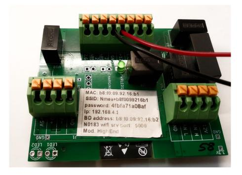
2. The ULP's cables will need to be connected to the top terminal of the plaque as seen in the picture. It is IMPORTANT to make a bridge between the GND of the ULP and the GND of the power source as is shown with the yellow arrows. We give power to
