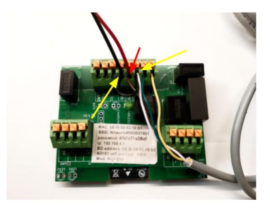
5. Wired Ultra-Low-Power RS485 wind sensor to NMEA1083 Display/Backbone
