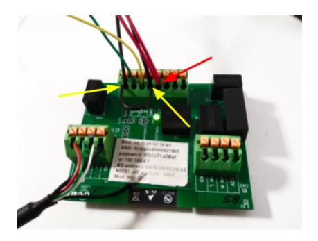
**3.** With this, we turn on the power source and confirm the **green light** is on. Now our NCP is configured to our wind sensor and connected to our display.
