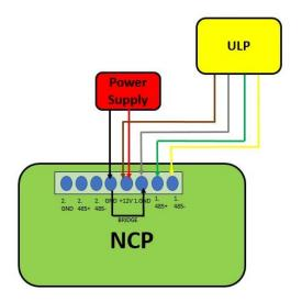
For the device to work, we will need to connect it to an external power supply of 12 Volts. The positive terminal of the energy source goes to the pin +12V of the ports of the top terminal as seen in the image. The negative terminal of the energy source connects to the GND. The green light should be lit. If it is not, check that the cables are properly connected. Before continuing any further, turn off the power to the energy source, do not disconnect the cables.
