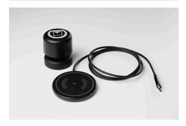
\*In order to check the battery charge level, connect to the Anemotracker App and the battery level is given on the main screen inside the compass. If there is no battery level shown, the device is not connected. Please **charge the device upside down** (as shown in the picture above) and then retry connecting to it via Anemotracker App. If it is connected, it will always show a level of battery.
