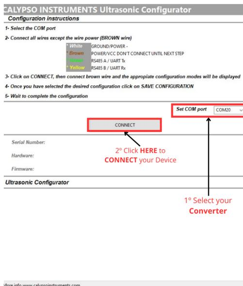
4. Connect the brown cable when the configurator tells you to.
