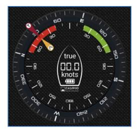
This shows the values of the Real and Apparent wind. The external circle is the compass, showing the north position (in degrees). The internal one is used by the Real and Apparent wind markers (red and yellow respectively) to show the direction from where the wind comes (in d e g r e e s ) .
