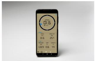
As you can see above, the app shows the Wind Speed (in this case in meters/second) and the direction degree. This direction degree means in which direction is the wind coming from taking the reference the **north mark** of the Anemometer. These two variables come from the Anemometer.
