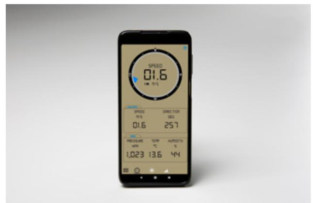
As you can see above, the app shows the Wind Speed (in this case in meters/second) and the direction degree. This direction degree means in which direction is the wind coming from taking the reference the **north mark** of the Anemometer. These two variables come from the Anemometer.
