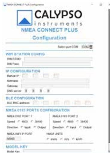
To configure the Portable wind meter to the NCP High-End fill in the following fields:
